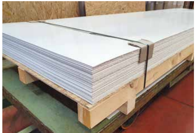
Made-to-measure standard pallet with continuous wooden surface
